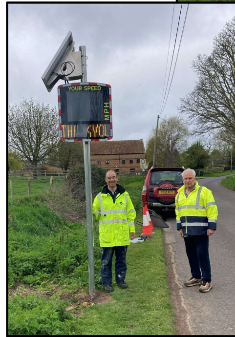
New SID (Speed Indicator Device) with solar panel
